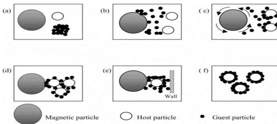
**Fig 2:** Mechanism of coating in the MAIC process: (a) excitation of magnetic particle, (b) de-agglomeration of guest particles, (c) shearing and spreading of guest particles on the surface of the host particles, (d) magnetic–host–host particle interaction, (e) Magnetic–host–wall interaction and (f) coated products.<sup>14</sup>
