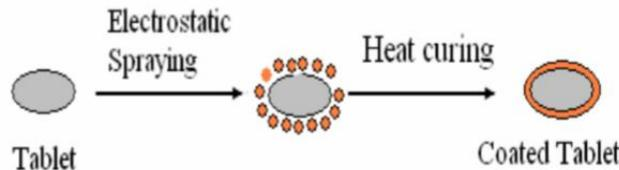
**Fig 1:** Mechanism of electrostatic coating.
