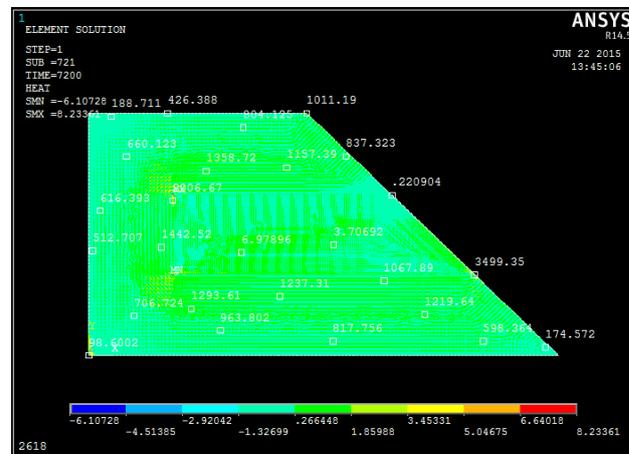
It can be observed that the largest magnitude of the thermal flow corresponds to the minimum point (MN) of the temperature distribution, because at this point the solidification begins.
